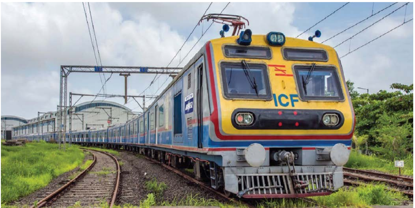
Air-conditioned AC-EMU manufactured for suburban railways
