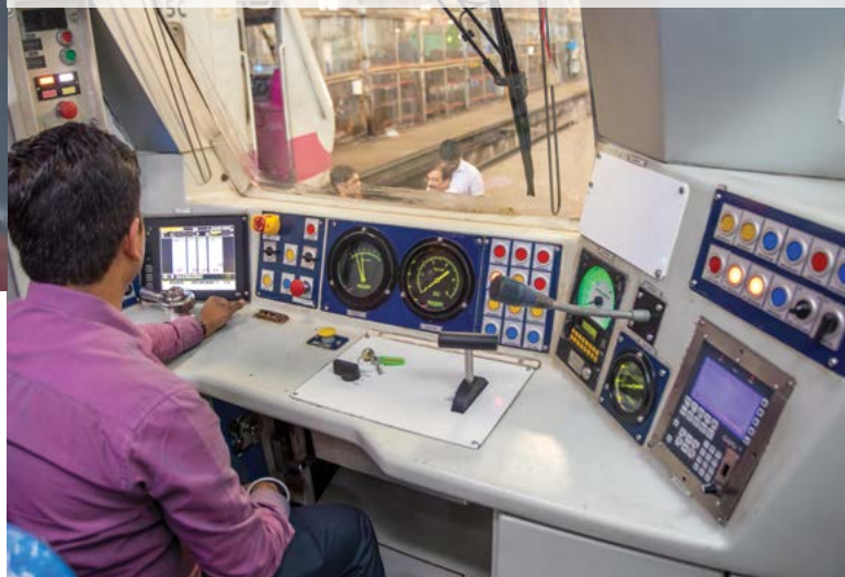
BHEL-make electrical & driver consoles inside AC EMU train
